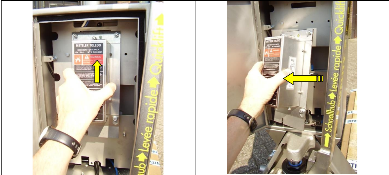
Lift up the battery pack slightly before taking it out.
